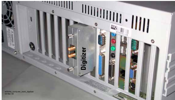
Figure 4 Connect adapter to back of PC digitizer card
