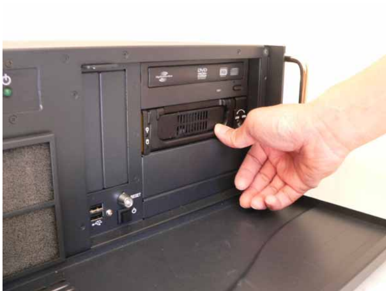
Figure 40 Ejector Lever Pushed Down
