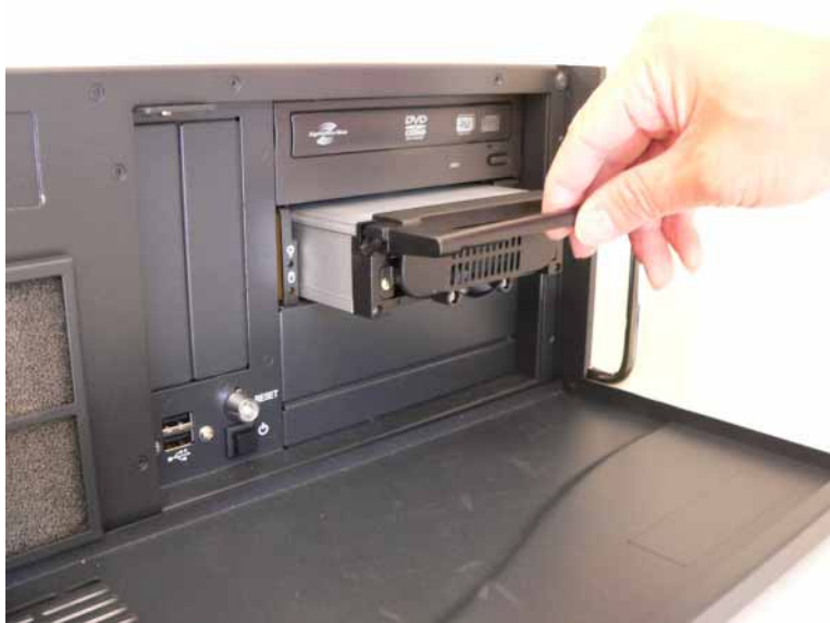
Figure 39 Ejector Lever Pulled Up
